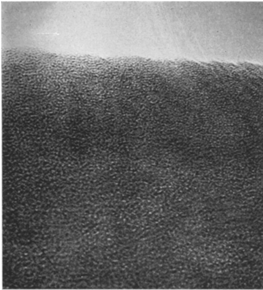
Figure 3 High resolution lattice image electron micrograph of non-crystalline phase in splat-quenched Al-17.2 at. % Cu ( \times 250000 ).
